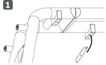
Access the wires in the tower. Be careful pulling out the wires. Next carefully cut the shrink wrap to uncover the wires. Be cautious not to cut through the wire insulation.
