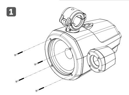
NOTE: disassemble the speaker on a clean flat surface to prevent scratches.
