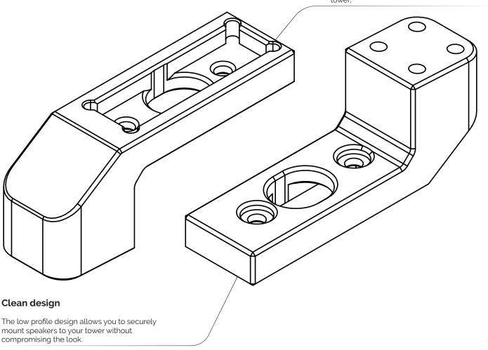
The F-Series Tower Speaker Adapters provide a solid platform to hang your speakers. Machined from billet aluminum it is sure to firmly hold your speakers for years to come.
