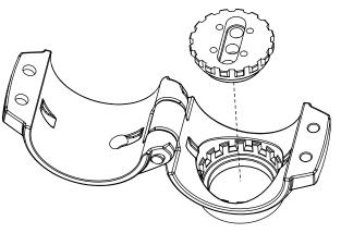
1: Insert the angle adjustment piece into the clamp base in the orientation shown.
