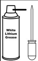
After the handle is installed, squirt some white lithium grease into the cam latch housing over the rotating parts of the cam latch.
