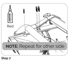
Install bolts and apply Red Loctite.
