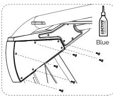
Step 5 Install bolts. Re-apply Blue Loctite.
