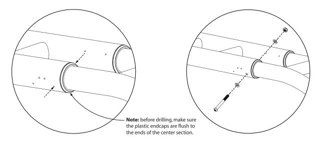
Once all 4 bolts are fastened, repeat drilling process for inside holes. Fasten all 4 inside bolts as illustrated.
