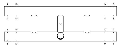
**Note:** We recommend inserting a bolt after each hole set is drilled (1,2; 3,4; etc.). This will reduce the risk of the tower moving out of alignment during the following sets of drilling.
