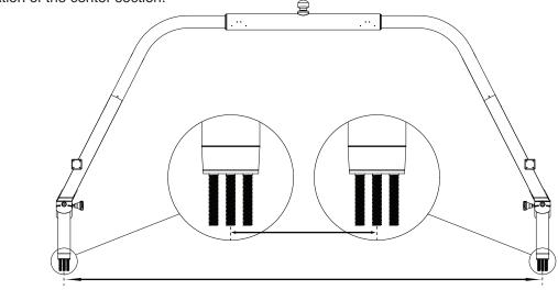
To make sure the center section is centered between the side sections, measure from the two tubes on each side as illustrated below. Once these two measurements are equal the center section will be centered.
