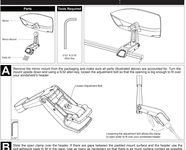
self-adhesive pads to fill in the gaps. Use as many as necessary so that there is as much surface contact as possible between the mount and the windshield header.
