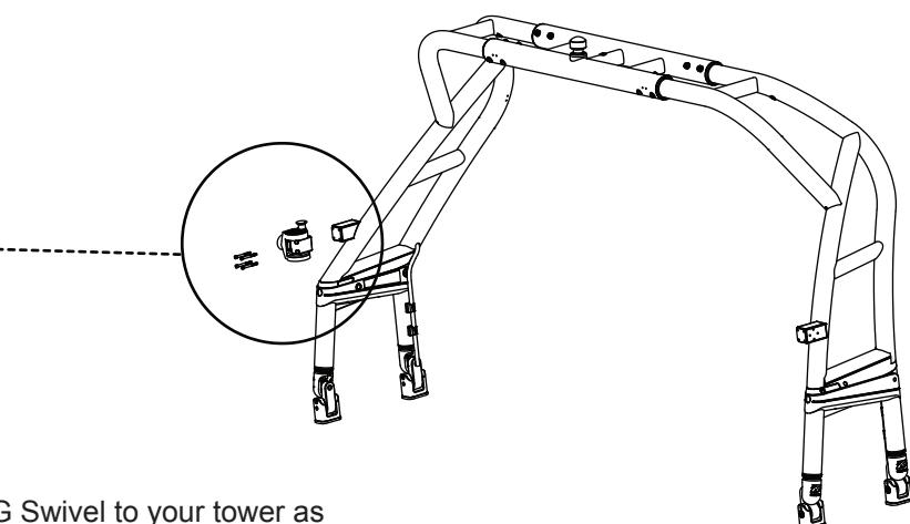
Assemble your MAG Swivel to your tower as illustrated with the Pull Pin facing up. Apply a small drop of red Loctite to each bolt prior to assembly.
