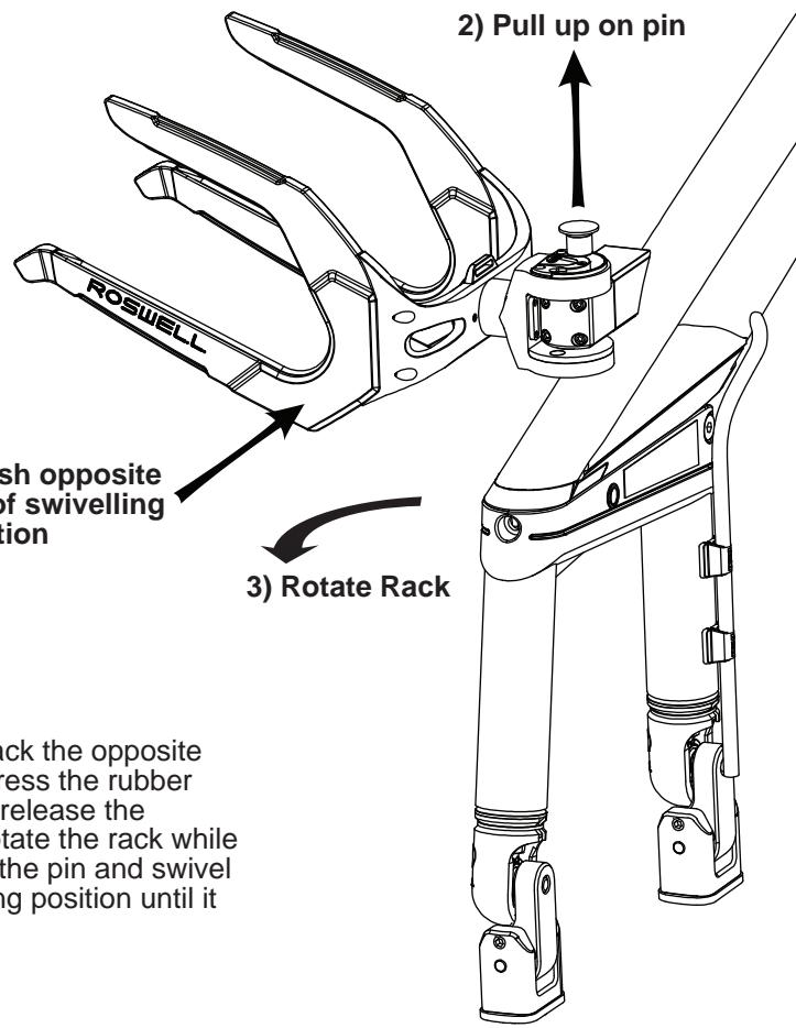
To use the swivel, 1) push the rack the opposite way you want to swivel to compress the rubber bumper. 2) Pull up on the pin to release the magnetic lock and 3) begin to rotate the rack while still holding the pin up. Release the pin and swivel the rack towards the other locking position until it locks into place.
