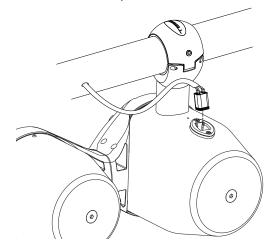
Loop the safety lanyard over the tower next to the speaker clamp.
