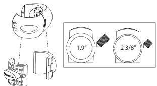
**Note** - To ensure tight fit use the correct plastic clamp inserts and set screws.
